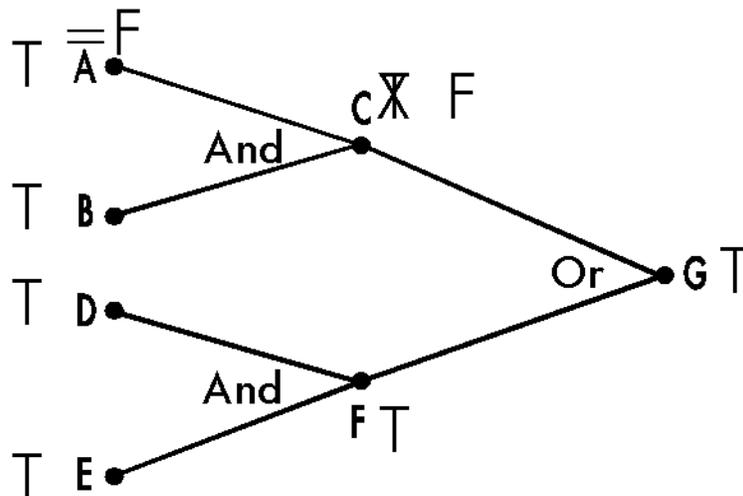
**Figure 5 - Variable "A" Stuck False Defect Not Observable**
