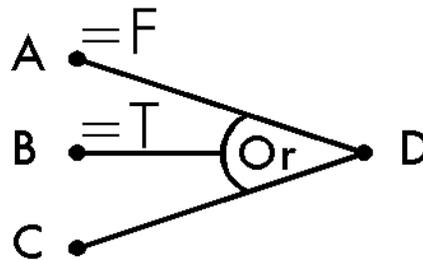
**Figure 1 - Simple "OR" Function With Two Defects**
